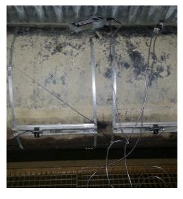
K1L sensors installed in a pair of mounting rails on the 950 mm grey cast iron pipe
